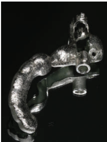
A printed titanium guide for a zygomatic implant
